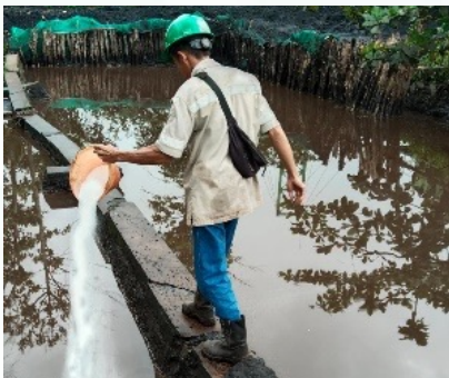
Pemberian Soda As di Settling Pond Sodium Carbonate Application in Settling Pond
